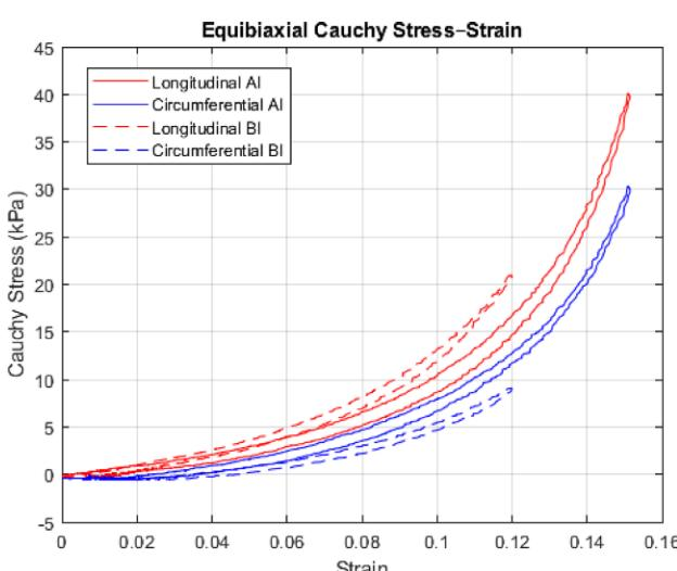
**Fig. 1** Equibiaxial Cauchy stress-strain responses for non-stented (NS) and stented (ST) samples
