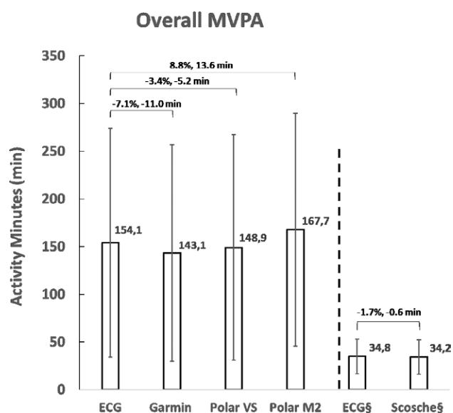
**Fig. 2** Volume of activity minutes each sensor recorded for the intensity zone moderate to vigorous physical activity (MVPA) compared to the ECG. Validity is considered high, if mean percentage difference is below 10%. Scosche has less data points since it was not used during the free-living phase due to its limited internal memory
